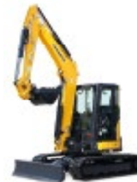
Crawler Excavator Vi055-6 Engine output: 33.4kW Max. digging depth: 3900mm
