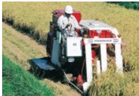
The TC1800 combine equipped with devices for automatic cutting-height control
