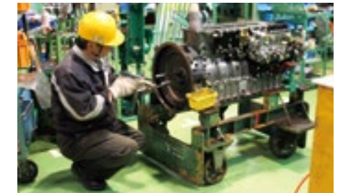
Cell manufacturing system at Tsukaguchi Plant
