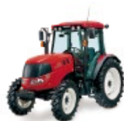
Diesel Tractors EG-PRO series Engine output: 48~105PS Weight: 2090~3595kg
