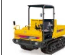
Crawler Carrier C30R-2B Engine output: 24.6kW Max. payload: 2500kg
