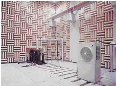
Noise level measurement in soundproof room
