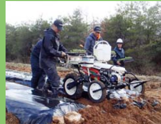
Transplanting cabbage by using a Yanmar-made NAPURA vegetable transplanter
